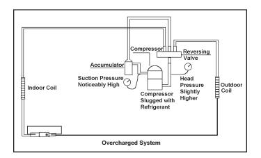
of the evaporator will not be encountered because the refrigerant will boil later if at all. Gauges connected to system will usually have higher head pressure (depending upon amount of overcharge). Suction pressure should be slightly higher.
